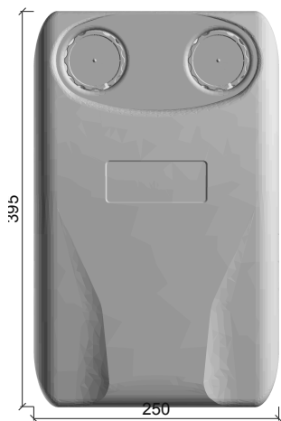
Fig. 3. EPP BLACK shell, dimensions in mm
