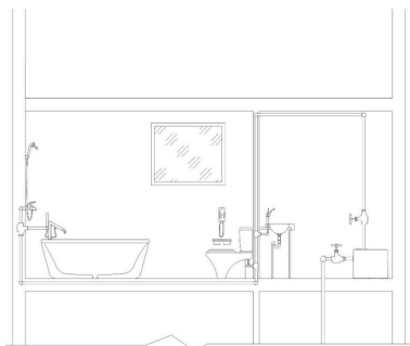
Fig. 2. Boosting the pressure of mains water.
