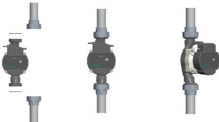
Fig. 8. Installation sequence: the pump goes between the union nuts, then the panel is turned to the required position
